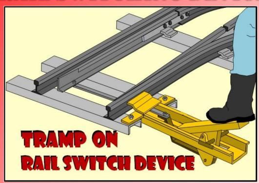
The switch point assembly ensures a simpler, <u>SAFER</u> and easier method of moving rail switch blades.
